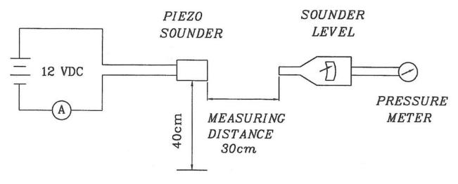
S.P.L. Measuring Circuit Mic: RION S.P.L. meter UC 30 or equivalent S.G.: Hewlett Packard 33120A Function Generator or equivalent
